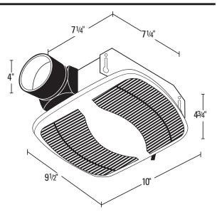
Acceptable for use over tub or shower when installed in a GFCI protected branch circuit.
