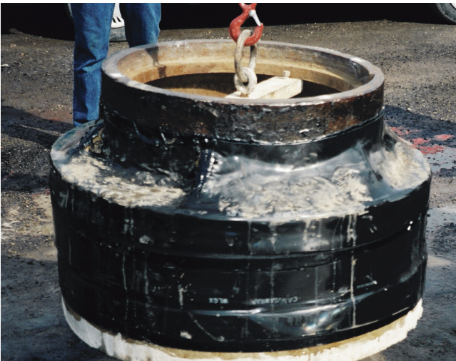
WrapidSeal™ adhesive strength demonstrated with vertical lift.
