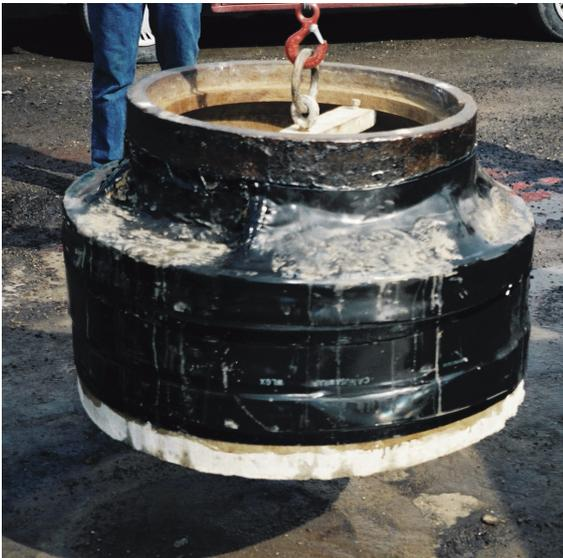
*WrapidSeal™ adhesive strength demonstrated with vertical lift.*
