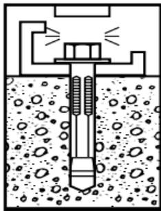
2. Insert assembled anchor into hole, so that washer or head is flush with materials to be fastened.
