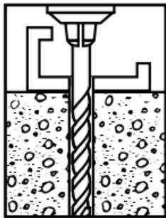
1. Use a bit with a diameter equal to the anchor. See selection chart to determine proper size bit for anchor used. Drill hole to any depth exceeding minimum embedment. Clean hole.
