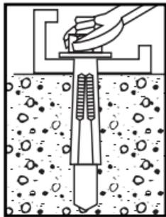
3. Expand anchor by tightening nut or head 2 to 3 turns.
