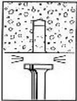
2. Drive anchor flush with surface of concrete.
