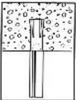
3. Expand anchor with setting tool provided. Anchor is properly expanded when shoulder of setting tool is flush with top of anchor.
