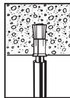
4. Expand anchor with setting tool provided (see chart). Anchor is properly expanded when shoulder of setting tool is flush with top of anchor.
