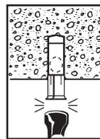
3. Drive anchor flush with surface of concrete.
