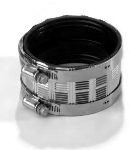
PIPECONX shielded couplings are elastomeric sleeves with stainless steel shields for use in joining cast iron, plastic, steel, copper and tubular in sewer and DWV systems.
