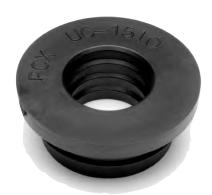
Use PIPECONX utility connectors to connect 1" or 3/4" CPVC and copper pipe to 1-1/2" DWV Schedule 40 plastic sockets (ABS or PVC) with a simple press fit. Our utility connectors are not for use in pressure water systems unless appropriate solvent cement is applied to the fitting socket and the utility connector.
