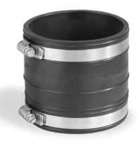
PIPECONX Expansion Joints are designed for vertical installation and allow for thermal expansion and contraction of drain, waste and vent (DWV) systems. The one-piece design saves you money by eliminating costly offsets. With no sliding parts to malfunction and an internal stop for positive positioning, you can be assured of a maintenance-free connection.
