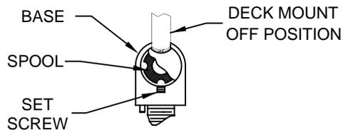
UNIT IS SHIPPED IN DECK MOUNT CONFIGURATION. TO CONVERT TO WALL MOUNT CONFIGURATION, POSITION ARM IN "DECK MOUNT OFF POSITION" AS ABOVE.
