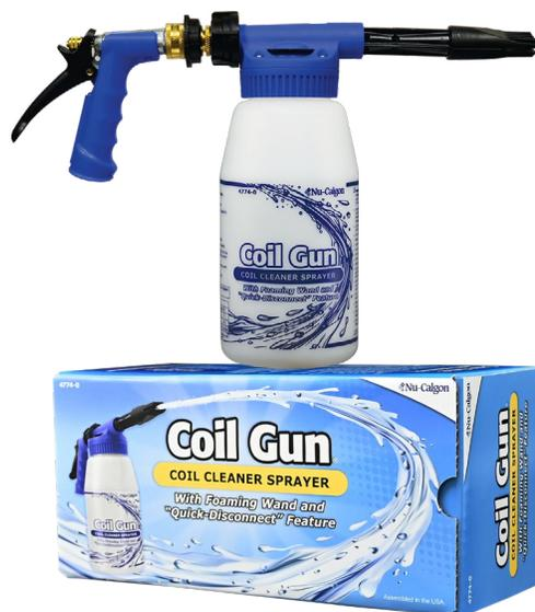
Turn dial to desired mixing rate letter to siphon chemical at the specific ratio. This will automatically mix chemical with water at the factory pre-set dilution rate selected on dial. When using Nu-Calgon's Ultra Concentrate product, sprayer must be used at 10:1 (setting E). Pistol grip shut-off-valve lever must be fully depressed for accurate mixing.
