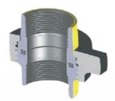
C&C's Figure 300 is manufactured from carbon steel. This Flat-Face type union has an O-Ring seal. Recommended for use where straight breakout of pipe segments is required. Suitable for water, oil, or gas service at pressures up to 12,500 PSI NSCWP. Please note that colors vary per pressure rating.
