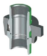
C&C's Figure 1003 (Mis-aligning Union) has NPT or Butt Weld Ends. It is constructed of Forged Alloy Steel, and comes with a Buna N O-Ring. Recommended for high pressure water, oil, mud or gas service where alignment of piping is a problem, with up to 7 1/2° angular adjustment from center (15° total).
