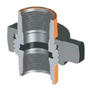
C&C's Figure 602 has a replaceable lip-type seal ring of Buna-N specifically designed to minimize fluid flow turbulence. The replaceable lip-type ring also provides a pressure seal and protection for the metal-to-metal seating surfaces. These unions are recommended for manifold and truck mounting where size and weight are critical. Recommended for air, water, oil, gas or mud service up to 6,000 PSI NSCWP.
