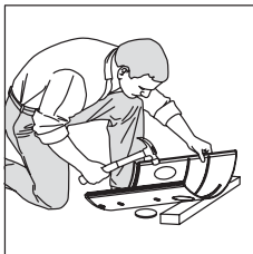
1 Knock out ports as needed from inside of panel
