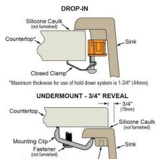
Feature for Top Mount version ' (not used in Undermount model) Designed to affix to the underside of any solid surface countertop.
