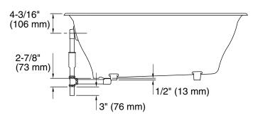
No change in measurements if connected with drain illustrated. (K-7145)
