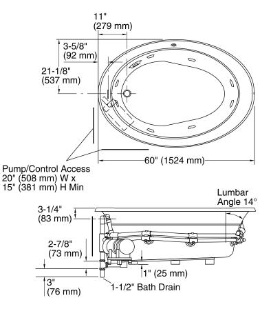
No change in measurements if connected with drain illustrated. (K-7166-AF)
