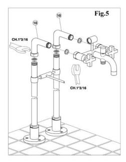
Screw the floor pillar legs to the inlet water connections: make sure that these are G. 1/2" male threaded and keep them at a range of 5"29/32 (see fig.1).
