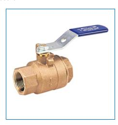
**Specifications UPC** Code 039923675323 Type Ball Valve T -- Female NPT Thread (FIPT) **Connection Type** Valve Size 2 Material Bronze CS Standard Lever Handle **Valve Operator** T58070 2 THRD BALL CONV PT BRZ **Description** eClass Classification Bronze Ball Valves All Type of Item Valve **Valve Pressure Rating (SWP)** 150 PSI / 10.3 Bar SWP **Turns/Operation** Quarter-Turn
