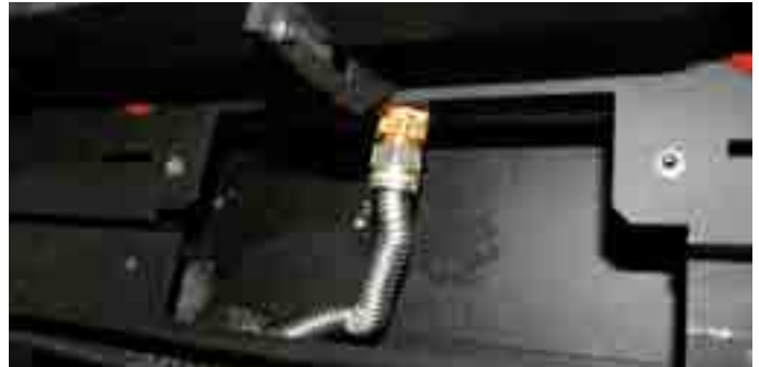
Figure 36d. Disconnect the flexible gas connection line.
