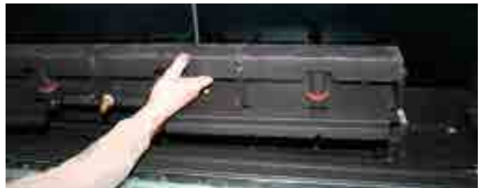
Figure 36e. After removing the appropriate fasteners, remove the burner assembly.
