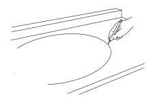
Measure and compare the thickness of the lavatory rim and tile. The lavatory rim thickness is 3/8" (1cm) +/-1/32" (1mm). Because of the varying thickness of the tile and lavatory, or if adhesive or mortar bed installation is used, make allowances to shim the lavatory, or route the underlayment as required.
