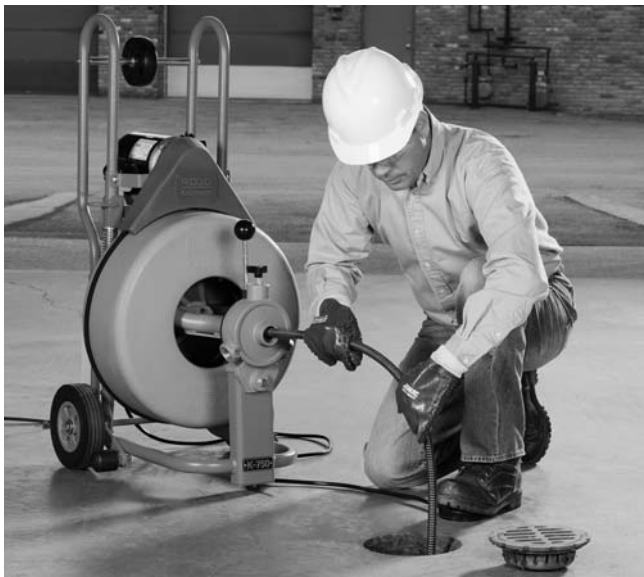
Figure 12 – In Operating Position, Manually Feeding Cable
