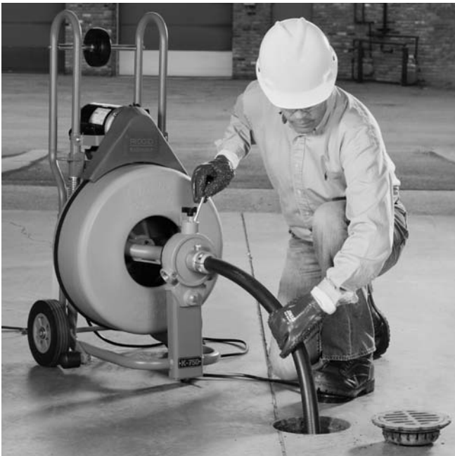
Figure 15 – Using Machine with Guide Hose
