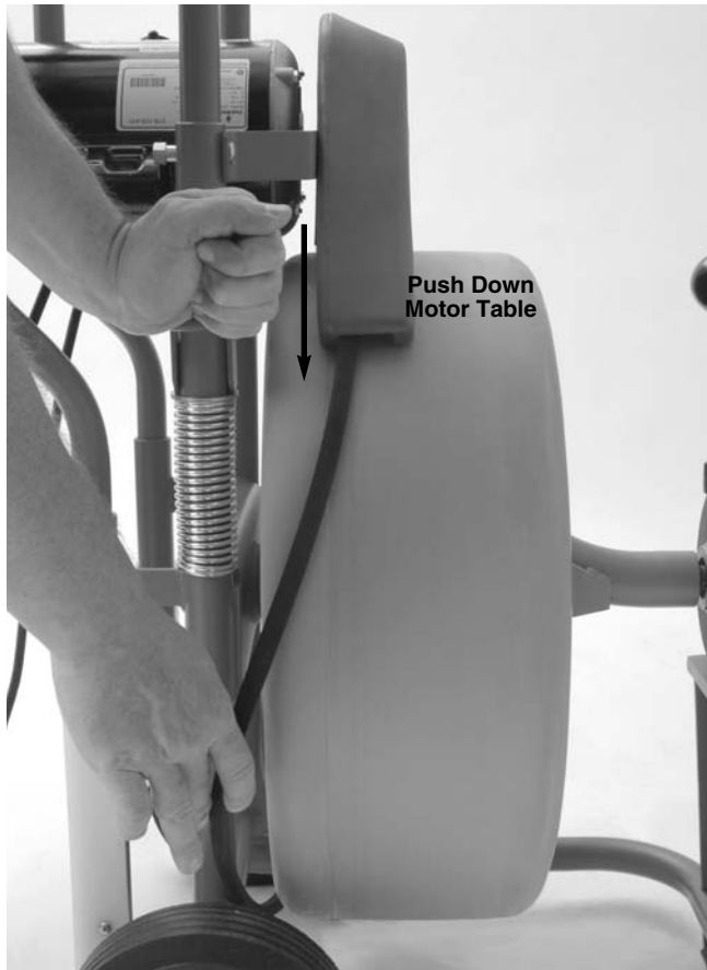
Figure 17 – Releasing Belt Tension
