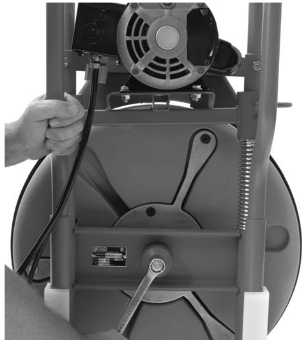
Figure 18 – Removing Drum Bolt
