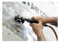
Cutting through panels is easy and accurate using Dynabrade cut-off tools. Powerful air motors drive abrasive wheels efficiently, and the variety of formats - straight, offset, right angle - allow operators greater control in their application.
