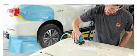
Dynabug® sanders are an ideal choice for use in feather edging applications. The square pad and delicate orbital motion allow technicians to sand in corners without undercutting. When equipped with a long-nap pad and non-woven nylon abrasives Dynabug® and Dynabug® II sanders are excellent scuffing and blending tools.
