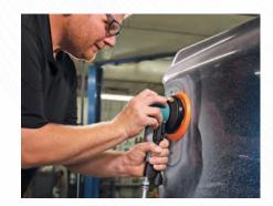
The DynaLocke® quickly strips paint to bare metal when set to rotary mode and converts to random orbital to complete the feather-edging portion of the application.
