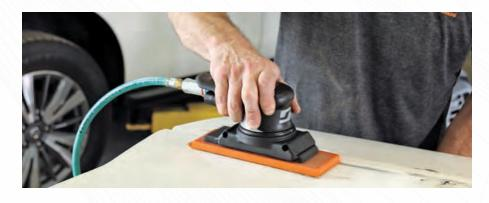
The in-line sanding motion of a Dynaline sander provides technicians with a powered option for completing traditional hand blocking applications. When used with non-woven abrasives Dynaline sanders are a great option for scuffing and surface preparation applications.
