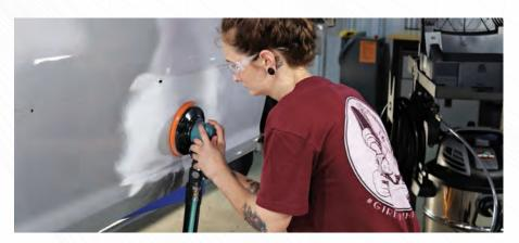
The Dynorbital-Spirit® is the lightest random orbital sander from Dynabrade and is ideal for vertical feather-edging applications where technicians are working in front of their body or at eye level with a vehicle raised on a lift. Weighing less than two pounds the Spirit sander reduces operator fatigue and relieves stress on wrists and arms. Improve shop air quality by combining with Dynabrade Mini-Raptor Vacs®.
