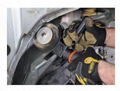
When equipped with a wire wheel the Dynabrade Nitro Series<sup>™</sup> NitroZip removes seam sealer quickly and without clogging leaving the surface below ready for rework.
