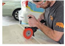
Using an eraser wheel the Dynabrade Nitro Series™ NitroZip quickly removes decals without harming the paint below, as well as removing adhesives without smearing on the painted surface.
