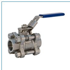
**Specifications UPC** Code 039923794116 Type Ball Valve **Valve Size** 1 1/2 T -- Female NPT Thread (FIPT) **Connection Type** Seal Material RPTFE (Reinforced) **Seat Material** RPTFE (Reinforced) Stem Material SS - Stainless Steel **Ball Material** SS - Stainless Steel **Body Material** Stainless Steel Cv Coefficient 143 **Valve Operator** CS Locking Lever Handle
