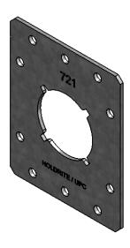
The PEXRITE® #721 is a 14 gage galvanized steel bracket that integrates directly with the PEXRITE® #701 Clamp, #704 Insert and HOLDRITE Stout Brackets®. It provides a PEX pipe support solution for lavatory and toilet applications. The #721 also attaches directly to wood, metal or concrete and various HOLDRITE® #100 and #400 series inserts.
