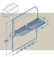
\*Optional backsplash is recommended when using infrared heat lamp
