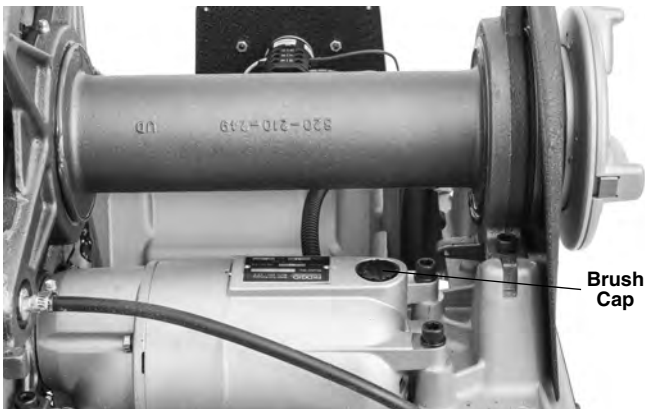
Figure 34 – Removing Motor Cover/Changing Brushes
