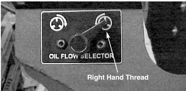
Figure 24 – LH or RH Oil Flow Selector
