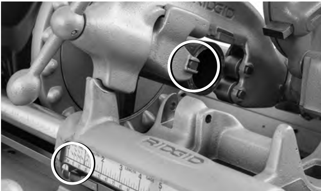
Figure 20A – Cutter Wheel Blade Against End of Pipe. Set Pointer to Zero (0)
