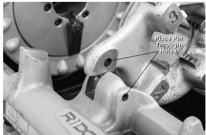
Figure 26 – Retaining LH Die Head in Place
