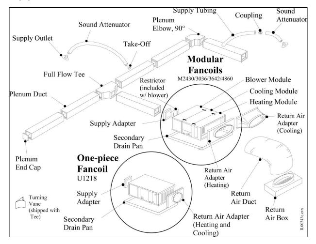
Figure 1. Air Distribution System Components (fiberglass duct board plenum shown)
