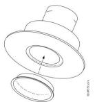
Figure 7. Installing winter shutoff caps
