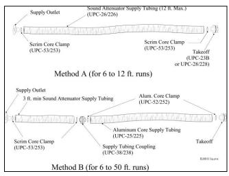
Figure 2. Brand Duct Assembly
