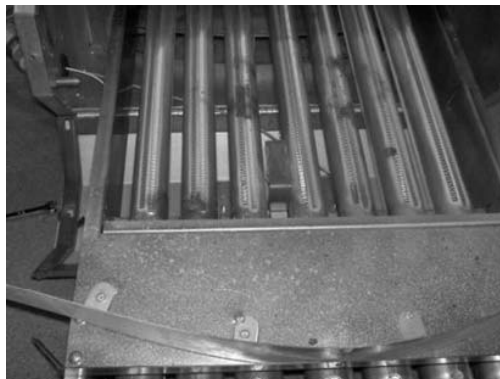
Step 14: Slide out burner assembly
