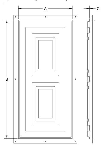
**Engineering Specification:** PEX QKPanel Manifold Access Panel allows access to the manifold after installation. The white ABS frame and door are lightweight and durable. The access panel has a lift-out door and stay-in-place frame. The 14" wide opening allows easy access to the manifold and connections.
