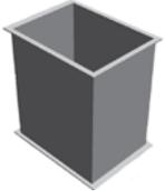
Constructed of fiberglass with an integral fiberglass anti-flotation flange. Designed to house the valves eliminating the need to enter the wet-well for service work. Available with or without discharge piping and valves.
