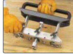
Outer rollers may travel off material and easily back on to complete bend because two roller stations can remain aligned on the edge of material.
