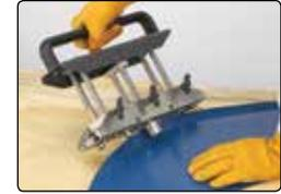
Also adjusts for making curved bends. The center roller station is independently adjustable, with the outer roller stations retracted and locked, to allow for bending on a slight curve.
