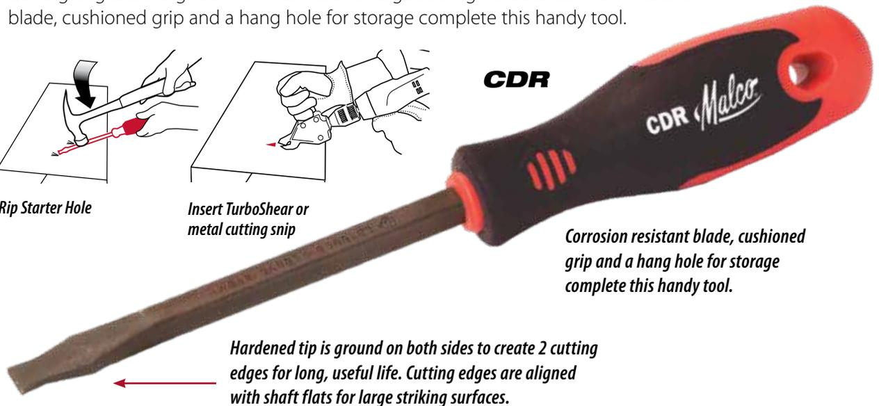
**Corrosion resistant blade, cushioned grip and a hang hole for storage complete this handy tool.**
