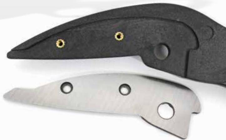
**Worry-Free Blade Changes!** Malco Ultra Lightweight Snips utilize a fully threaded brass insert thermally anchored in the blade area of the polymer frame for holding power and no loss of thread integrity.
