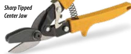
**The Max2000 Double Cut Snip** employs a best of all worlds close tolerance design for consistent performance. A curved cutting edge on the center jaw reduces cutting force required and large relief grinds on all jaws minimize drag. The double cut blades feed smoothly, cut cleanly without surface distortion, and easily navigate metal seams encountered in round metal duct and stove pipe. A self-starting point on center jaw makes short work of blind cuts.
