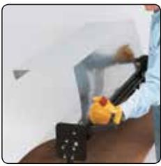
Accommodates sheet metal up to 48 in. (1.2 m) wide in any length. There is no fixed throat depth to contend with.
