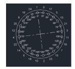
7. Hand tighten each actuating bolt in a clockwise direction until contact is made between each wedge insert and the pipe OD. Continue tightening the actuating bolts in an alternate method (STAR PATTERN) until all the break-off tops have been removed. Never tighten actuating bolt more than 180 degrees before moving to the next bolt.
