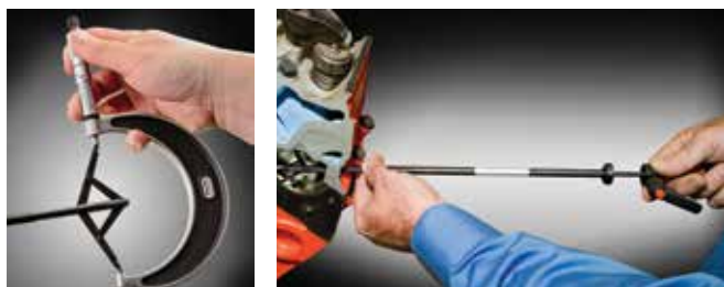
Cylinder Gage - custom built for Porsche
