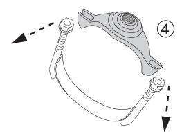
Step 5 • Position the saddle body on the pipe. Do not slide saddle on pipe.
