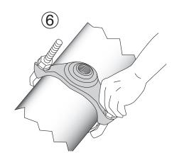
**Step 7** • Tighten all nuts evenly in 15-20 ft-lbs. increments. Keep bolts tight to the body. Use a wrench with at least a 12 inch handle.
