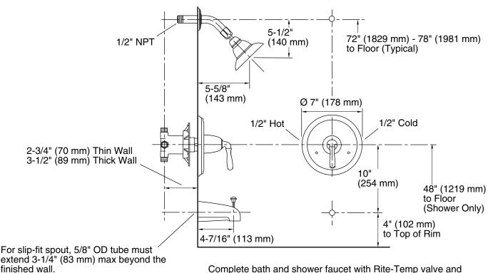
extend 3-1/4" (83 mm) max beyond the finished wall. For 1/2" NPT spout, pipe must extend 3-5/8" (92 mm) beyond the finished wall.
