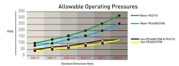
NOTE: Operating Pressure for Conventional Tapping Tees and Conventional Branch Saddles are determined by the material used, the outlet SDR and the governing regulations.
