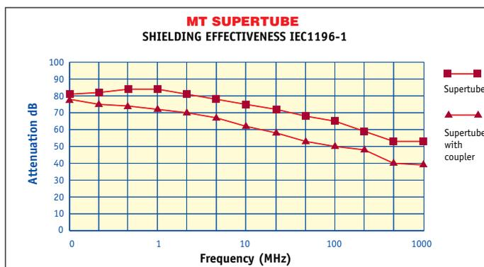
The graphs above show that the shielding effectiveness of MT Supertube is highly effective throughout the entire frequency range and will provide protection from interference for data, telecoms and signal cables.
