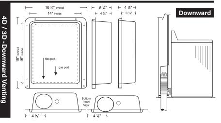
Model Wall **Exhaust** Number **Size** Direction DB-480 2X6 Up & Down Upward DB-425 2X6 DB-350 2X4 Upward DB-4D 2X6 Downward DB-3D 2X4 Downward
