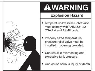
This water heater is provided with a properly rated/sized and certified combination temperature-pressure relief valve (T&P valve) by the manufacturer. The valve is certified by a nationally-recognized testing laboratory that maintains periodic inspection of the production of listed equipment and of materials as meeting the requirements for **Relief Valves for Hot Water Supply Systems, ANSI Z21.22 · CSA 4.4**, and the code requirements of **ASME**.
