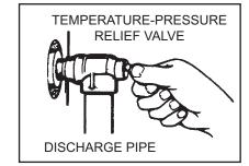
Figure 11. Temperature-Pressure Relief Valve Test
