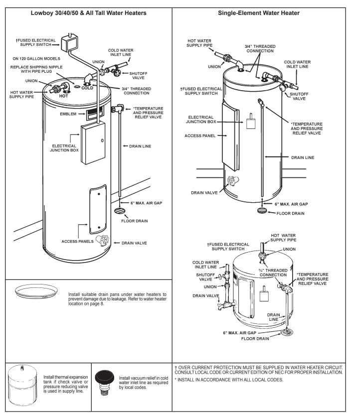
Figure 4. Typical Water Heater Installations
