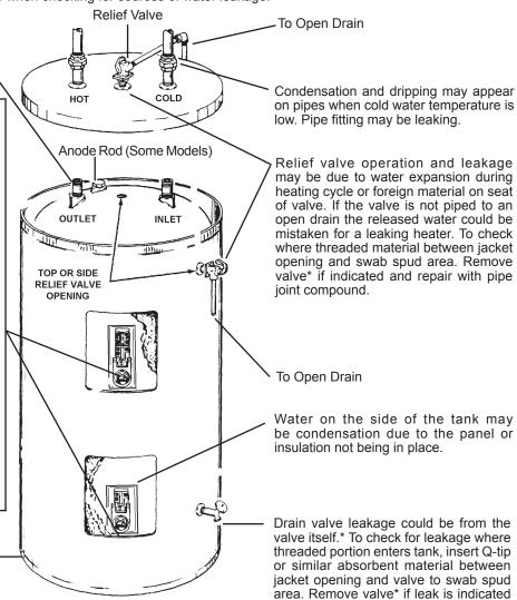
shut off electricity and drain tank to perform procedure.
