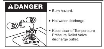
It is recommended that the temperature-pressure relief valve should be checked to ensure that it is in operating condition every six months.
