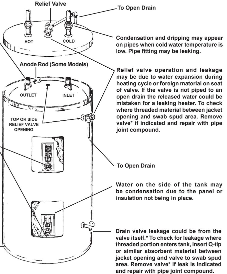
\*Contact your dealer as it is necessary to shut off electricity and drain tank to perform procedure.
