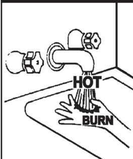
Water temperature over 125°F (52°C) can cause severe burns resulting in severe injury or death.
