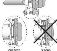
Care must be taken to assure that the flanges of the gland and MJ fitting remain parallel during the entire installation.
