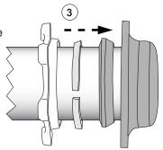
**Step 4** • Slide the gasket into the MJ bell pocket as far as possible. The gland (and GripRing) may be used to tap the gasket into place if required. Be sure that the gasket is properly seated and fully pressed into the gasket recess.
