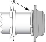
Step 6 • Slide the gland up the pipe until it engages the GripRing.
