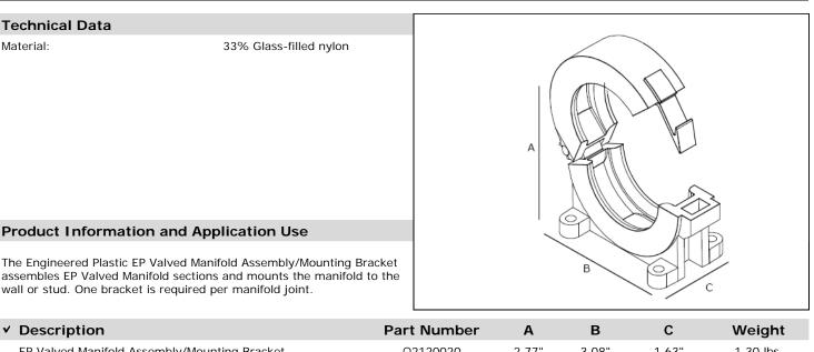
The Engineered Plastic EP Valved Manifold Assembly/Mounting Bracket assembles EP Valved Manifold sections and mounts the manifold to the wall or stud. One bracket is required per manifold joint.
