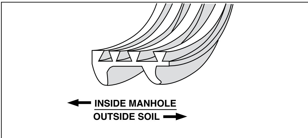
**Step 1** • Check the area where gasket will seat on the pipe to make sure there are no dents, projections, gouges, etc that will interfere with the gasket seal. Welds must be ground flush.
