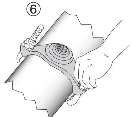
**Step 7** • In 15 - 20 ft-lbs. increments, tighten nuts to 30 - 35 ft-lbs. Keep bolts tight to the body. Use a wrench with at least a 12 inch handle.
