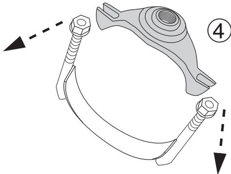
**Step 5** • Position the saddle body on the pipe. Do not slide the saddle on the pipe.
