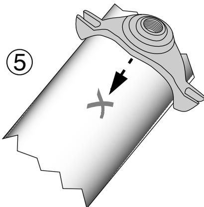
**Step 6** • Install strap(s) on saddle body, and tighten finger tight. Make sure the gasket has seated itself flat onto the pipe face.
