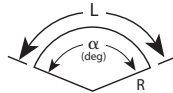
Sector of Circle A = \pi R^2 \frac{\alpha}{360} L = \pi R \frac{\alpha}{180} \alpha = 57.296 \frac{L}{R} R = 57.296 \frac{L}{\alpha}
