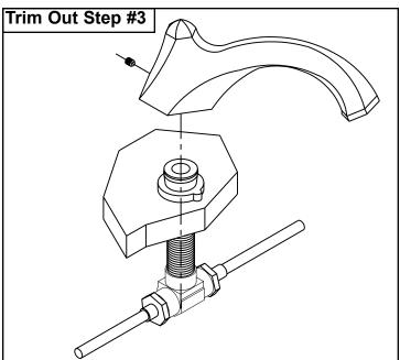
Set the deck spout onto the quick connect spout adapter and tighten the set screw at the base of the spout with the supplied allen wrench.
