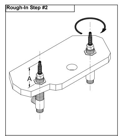
Connect the hot and cold supply piping to the 3/4" NPT at the bottom of the hot and cold valves.
