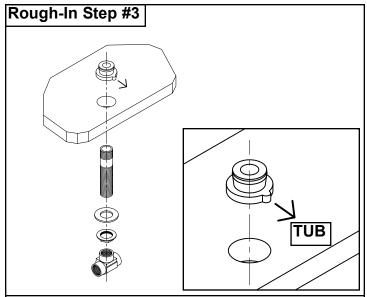
Apply teflon tape or pipe joint compound to the short end of the 3/4" spout nipple. Thread short end of the nipple into the quick connect deck spout adapter. Install the quick connect adapter through the 1-1/4" hole in the deck making sure that the deck spout adaptor sits flat on the finished deck.
