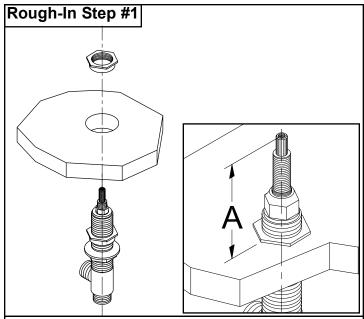
Insert the hot deck valve from below through a 1 1/2" hole and install the top-fastening nut. Set the deck valve to proper rough-in height by adjusting the top mounting nut and secure the valve by tightening the bottom valve nut. The rough in measurement is found by using measurement 'A' on the Rough In Specification sheet on the back of this pamphlet. The trim product number must be known. The stem and nipple may be trimmed to arrive at the correct rough-in measurement.
