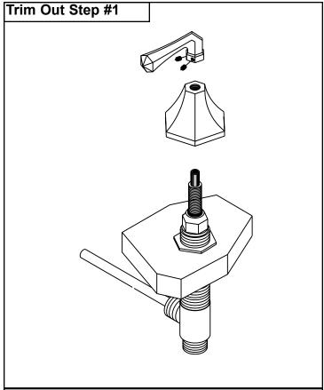
Attach the trim components by installing the escutcheons onto the valves. You may need to trim the nipple and stem.
