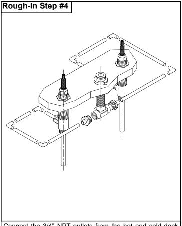
Connect the 3/4" NPT outlets from the hot and cold deck valves to the spout tee
