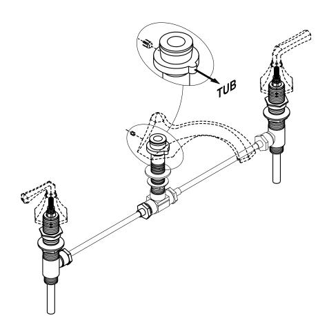
Valve shown: "A" Rough In Specifications "A" SNAP-ON INSERT 80001248 FOR DECK SPOUT IF YOU DO NOT KNOW THE TRIM NUMBER INSTALL THE VALVES AT A 2 5/8" ROUGH IN MEASUREMENT. 90001248 (NOTE: THIS IS THE DISTANCE FROM THE FINISHED **DECK TO THE TIP OF THE STEM.)** TO TUB TOP VIEW FINISHED DECK **DECK THICKNESS** 3/4" Min 3 <u>1/4"</u> Max FROM FROM VALVE TO SPOUT **VALVE** TO SPOUT 3/4-14NPT 3/4-14NPT FROM **FROM HOT SUPPLY COLD SUPPLY**
