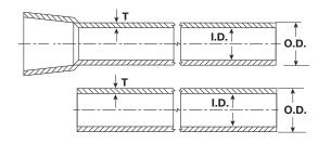
T: (Wall Thickness) O.D.: (Outside Diameter) I.D.: (Inside Diameter)
