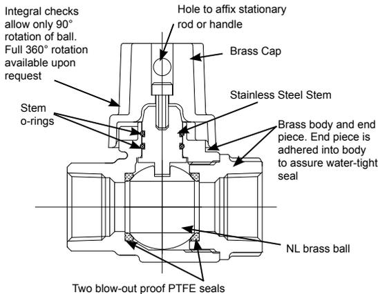
Cambridge Brass Ball Valve Curb Stops maintain their low turning torques and bubble-tight 300 PSIG water pressure rating due to the NL coated brass ball that is supported by two PTFE seals. Cambridge Brass Ball Curb Stops offer positive shut-off from either direction.
