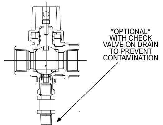
Cambridge Brass' Stop and Drain Ball Valve Curb Stops maintain their low turning torques and bubble-tight 300 PSIG water pressure rating due to the NL coated brass ball that is supported by two PTFE seals. Cambridge Brass Stop and Drain Ball Curb Stops offer positive shut-off from inlet direction only.
