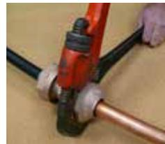
**4. TIGHTEN THE NUT:** Using standard wrenches, tighten the nut to seal and grip the pipe.
