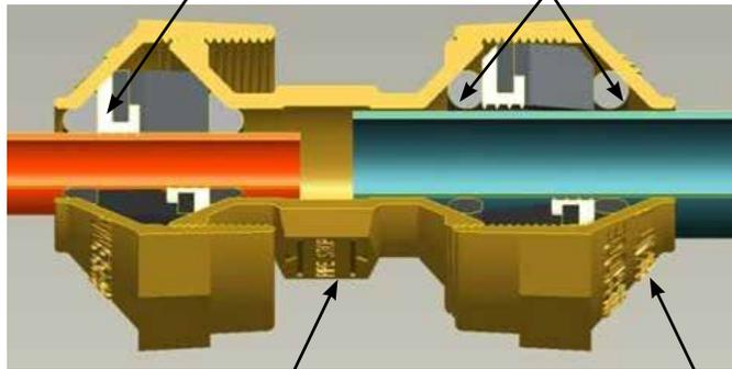
Pipes are inserted to the indicator markings on the body.
