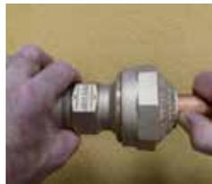
**3. INSERT THE PIPE:** Insert the pipe to the depth noted. (You may wish to tighten the nut to make the rubber close to the pipe diameter before insertion.)
