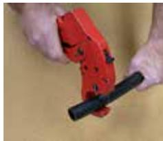
**1. CUT PIPE TO LENGTH:** Make a clean cut, square to the pipe using an appropriate cutter (roll cutter or shears are preferred.)
