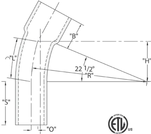
CANTEX Schedule 40 22-1/2-Degree Special Radius Belled End Elbows are used to change the direction of a conduit run by 22-1/2 degrees when special radiuses are needed.
