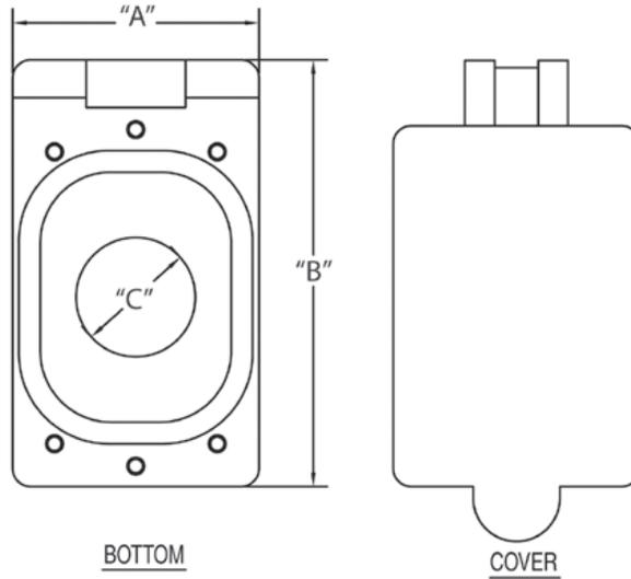
CANTEX 5133350 is a 1-Gang 15 Amp Weatherproof Receptacle Cover designed for use with exposed weatherproof boxes.
