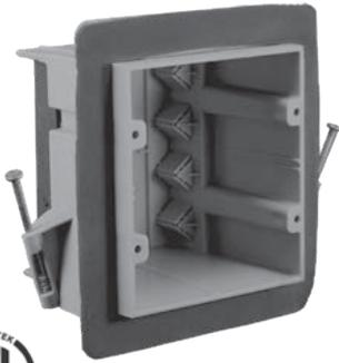
EZ36DN-RG is a 2-gang, new work, vapor-proof EZ Box. It is an energy efficient electrical box for walls subject to unwanted air-flow. It eliminates air leaks with a solid drywall flange covered with a foam gasket and additional foam gaskets over 8 self-clamping cable entry v-clamps, creating a vapor-tight seal preventing air from flowing through the box. The EZ36DN-RG also features angled nails for EZ secure installation.
