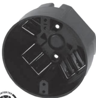
EZ20CZ deep ceiling fan box for (new work) new construction applications is a 20 cu. in. ceiling fan box. EZ20CZ is good for residential and light commercial applications. It features 6 wiring clamps for easy wire installation.
