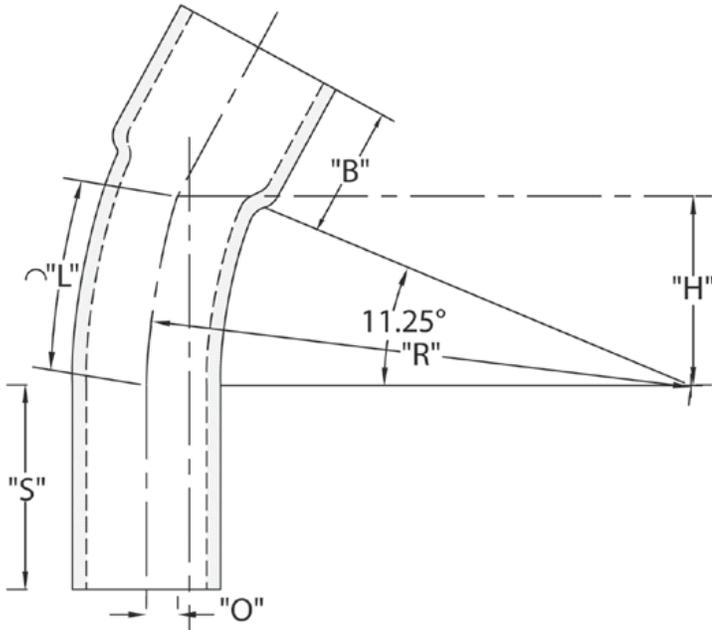
DB-60 Special Radius Bell End 11-1/4 Degree Elbows are used to change the direction of a conduit run by 11-1/4 degrees.
