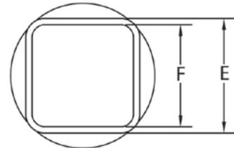
Telephone Duct Adapter - Adapts 4" Telephone Duct to 3-1/4" Round Clay Tile
