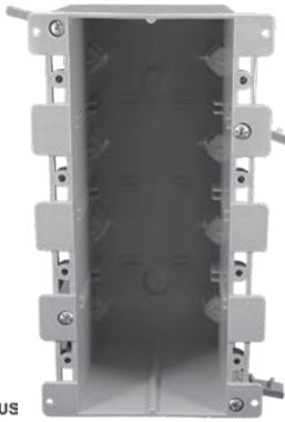
EZ68QO EZ BOX is a 4-Gang, 68 cu. in., renovation application (old work) electrical switch or outlet box for residential or light commercial renovation projects when a 4-gang box is needed. EZ mount flanges, winged swing tabs and built in wire clamps make installation easy and cost effective.
