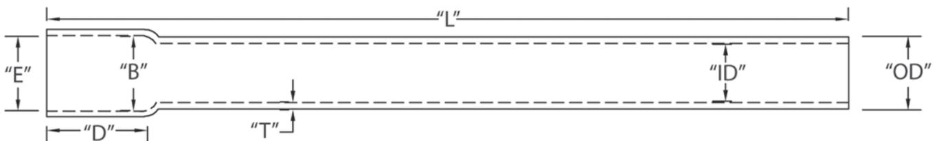
Note: 20' length available on request with the exception of the 1/2 and 3/4 conduit inch sizes. Schedule 80 conduit complies with federal and military specifications by conforming to UL 651. Call for special quotes.
