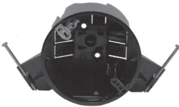
EZ25CNG-HW is a 25 cu. in., nail-on, heavy wall ceiling box for new work (construction) applications for residential and light commercial projects. It is a heavy duty new construction (new work) ceiling box to use where a more durable electrical box is preferred. The harder shell resists flexing and holds shape in extreme conditions. It features 5 heavy-duty wire clamps for EZ secure wiring. It features a ground lug for EZ grounding when required.
