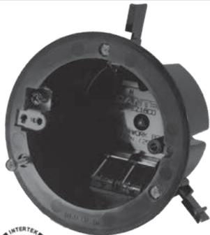
EZ18COG EZ BOX is an 18 cu. in., ceiling box with a ground lug for electrical ceiling applications for (old work) residential or light commercial renovation (old work) projects. The EZ mount flanges, wing tabs and built in wire clamps make installation easy and cost effective. CANTEX ceiling boxes are constructed with durable polycarbonate for added resilience.
