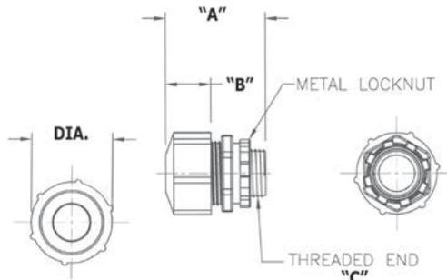
Strain Relief Connectors are designed to terminate a cable into a PVC box or enclosure.
