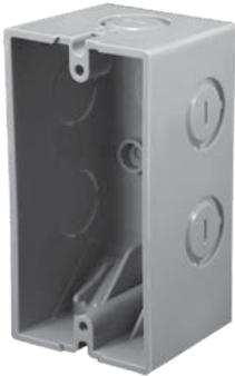
EZ12SO EZ BOX is a multi-purpose electrical switch and outlet box for residential or light commercial electrical installations, including switch, outlet, toggle switch and ground fault circuit interrupters. It features knockouts & 2 clamps for wiring and mounting versatility. Works with four CANTEX covers: EZSL-TGL Switch Cover, EZSL-DPLX Duplex Cover, EZSL-Blank, & EZSL-GFCI Receptacle cover.
