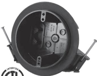
EZ26CN-RG is a new work, energy efficient vapor-proof ceiling box. It eliminates air leaks with a drywall flange covered with a foam gasket and additional foam gaskets over self-clamping cable entry v-clamps, creating a vapor-tight seal and allowing no air to flow through the box.
