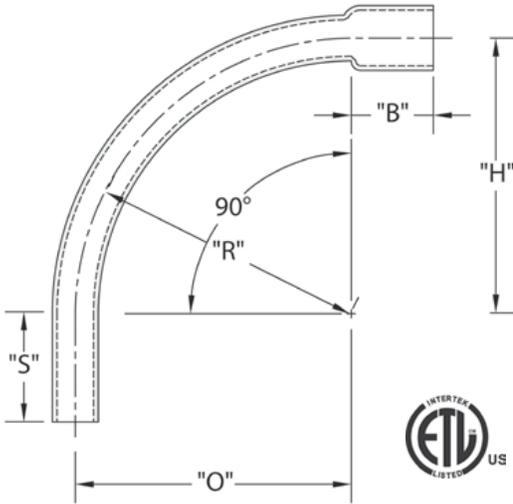
CANTEX Schedule 40 90-Degree Special Radius Belled End Elbows are used to change the direction of a conduit run by 90 degrees when special radiuses are needed.
