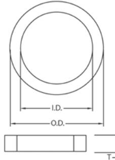
Sealing Washers or Rings are designed to be used with terminal adapters to provide a concrete tight connection.
