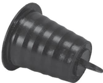
Poly Plugs with Pulling Eyes are designed for the temporary sealing of conduit to protect the duct from the effects of weather, job site debris, and animal damage. The molded in pull-eye is used to secure excess pulling rope within conduit.
