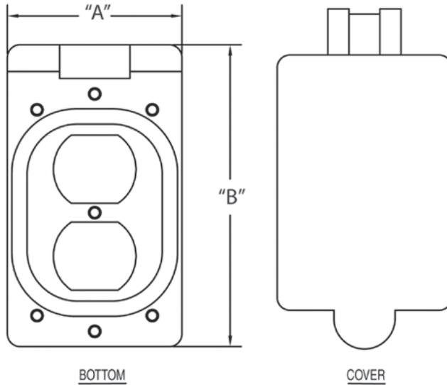
CANTEX 5133352 is a 1-Gang Weatherproof Duplex Receptacle Cover designed for use with exposed weatherproof boxes.
