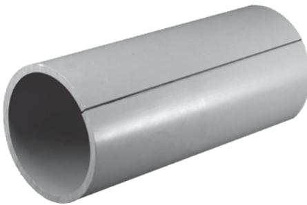
Schedule 40 Split Sleeve Couplings are used for joining Split Ducts to existing duct when repairing broken or damaged conduit and wires are present.
