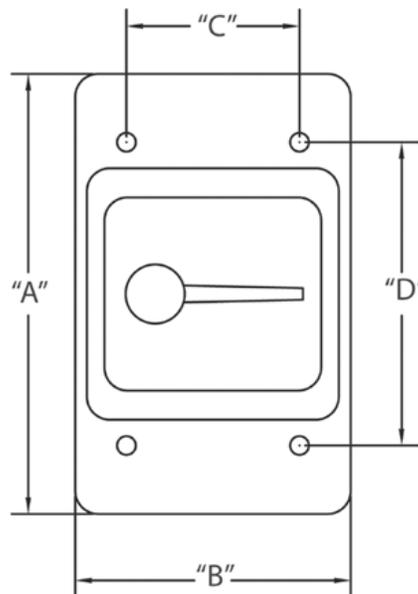
CANTEX 5133330 is a 1-Gang Weatherproof Toggle Switch Cover designed for use with exposed weatherproof boxes.
