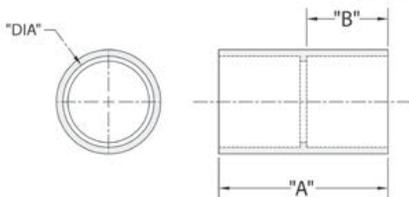
Schedule 40 Long Line Center Stop Couplings are used to repair or join lengths of conduit/ pipe together with two solvent weld socket ends.
