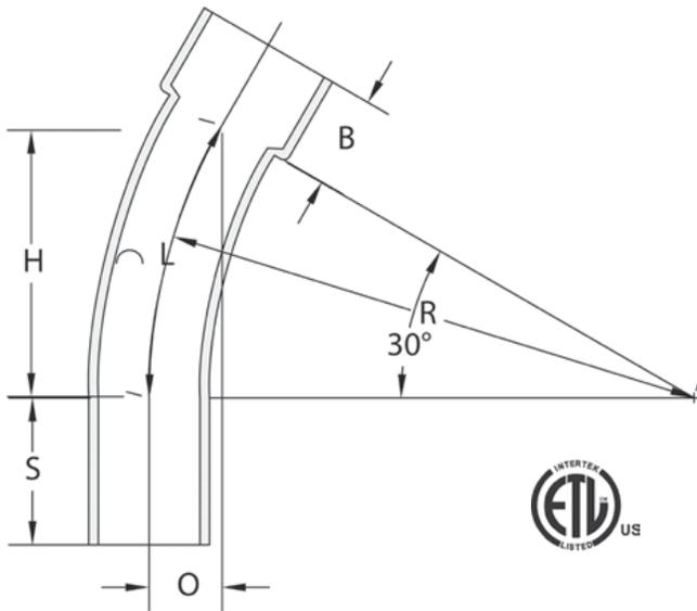
CANTEX Schedule 40 30-Degree Special Radius Belled End Elbows are used to change the direction of a conduit run by 30 degrees when special radii are needed.
