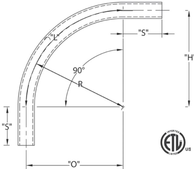
CANTEX Special Radius Plain End Schedule 40 90-Degree Special Radius Elbows are used to change the direction of a conduit run by 90 degrees when special radiuses are needed.
