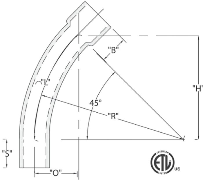
CANTEX Belled End Schedule 80 45-Degree Special Radius Elbows are used to change the direction of a conduit run by 45 degrees when special radiuses are needed.
