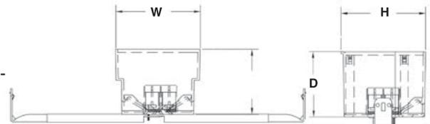
**EZ BOX® New Work, 20 cu. in. Ceiling Box with Hanger Bar, Wire Clamps and Ground Lug**
