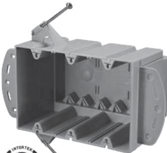
EZ74TNZU EZ BOX is a 74 cu. in., deep, 3-gang switch and outlet box for residential or light commercial new construction (new work) installations. It features molded brackets for steel stud mounting along with v-clamps, Express Clips® and screw-nails for EZ installation. The sharp point, slotted head and threaded body of screw-nails allow for installation with a power screwdriver without having to pre-drill aluminum, light to medium grade steel or wood studs.
