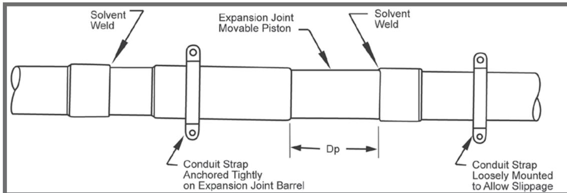
The correct piston setting,  $D_p$ , can be determined for any installation temperature by using the following equation:
