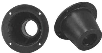
An ENT Stubby is used to create conduit stubdowns in concrete slabs. It gives protection to the ENT conduit from potential damage during the removal of wood forms.
