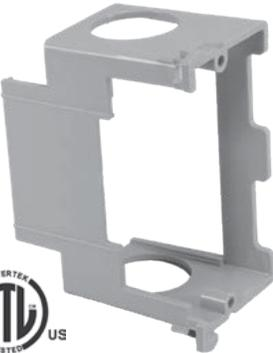
EZLVSB is a 1-gang, low voltage EZ BOX add-on bracket. It attaches to most non-metallic boxes to allow for low and high voltage applications side by side. EZLVSB is for both old and new work applications. The backless design is great for the large or deep low-voltage wiring needed for communications and cable installations. It fits most standard faceplates.
