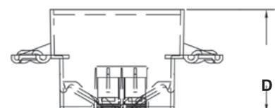
**EZ BOX® 20 cu. in., New Work, Nail-on Ceiling Box with Wire Clamps and Ground Lug**
