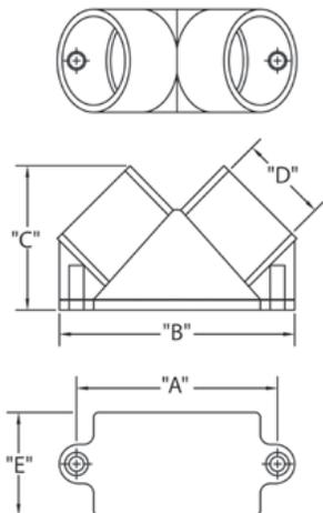
Pull Elbows are used to effect a sharp 90-degree turn in a conduit run where wires must be continuously pulled around the turn.
