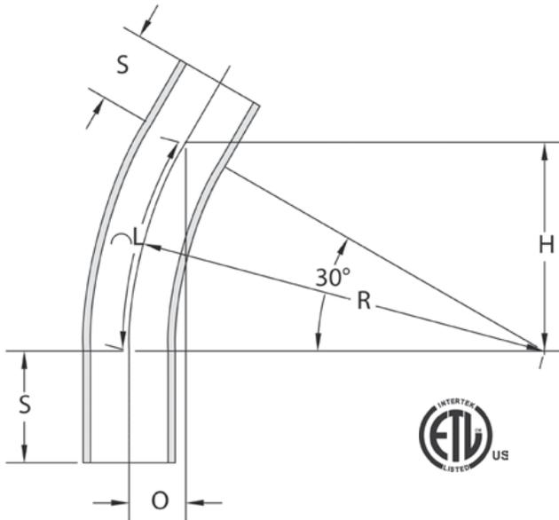
CANTEX Plain End Schedule 80 30-Degree Special Radius Elbows are used to change the direction of a conduit run by 30 degrees when special radii are needed.
