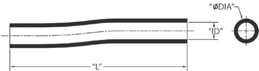
Conduit offset is a plain end section of conduit formed to go around obstacles or compensate for centerline differences in two conduit runs.
