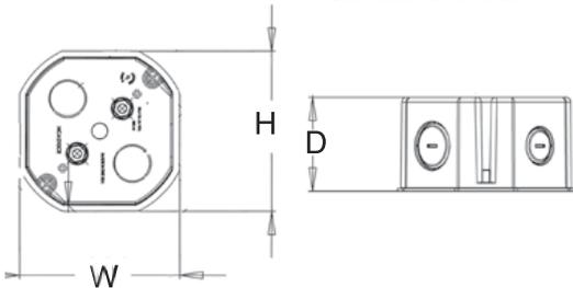
CANTEX EN20C is a 20 cu. in. Octagon ENT Ceiling Box for residential and light commercial ceiling fixture applications. It features 6 knockouts for multiple wiring options.
