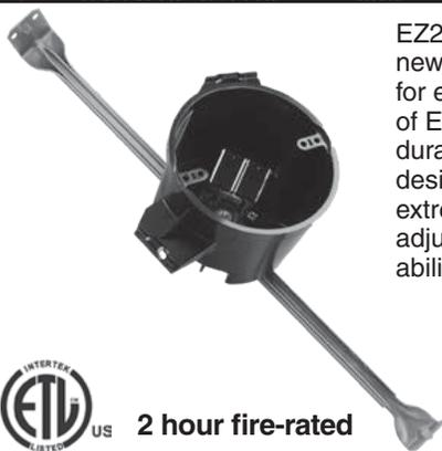
EZ25CH-HW EZ BOX is a 25 cu. in, heavy wall, new work ceiling box with an attached bar hanger for extra support and adjustability. The harder shell of EZ25CH-HW is designed to use where a more durable electrical box is preferred. The harder shell is designed to resist flexing and hold its shape during extreme conditions. The adjustable bar hanger adjusts from 14" to 18" for added support and adaptability. It also features 5 integral wire clamps.
