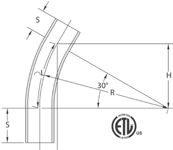
CANTEX 30-Degree Plain End Schedule 40 Special Radius Elbows are used to change the direction of a conduit run by 30 degrees when special radiuses are needed.
