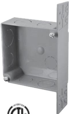
EN20DB is a 4 inch Square, 20 cu. in., ENT switch or outlet box designed for use with electrical nonmetallic tubing (ENT). 4" square boxes provide maximum volume for multiple conductors and connectors running in multiple directions. EN20DB features molded flanges and 7 knockouts for EZ installation and multiple connections.
