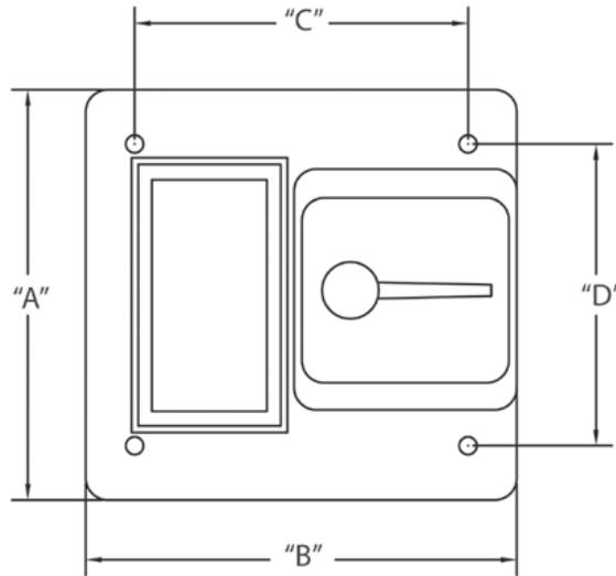
CANTEX 5133345 is a 2-Gang Weatherproof GFI & Toggle Switch Cover designed for use with exposed weatherproof boxes.
