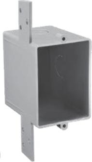
EN16SB is a 1-gang, 16 cu. in., ENT switch or outlet box designed for use with electrical nonmetallic tubing (ENT) and standard electrical devices and switches in residential and light commercial applications. EN16SB features a molded flange and three 1/2 inch knockouts for EZ installation and multiple connections.
