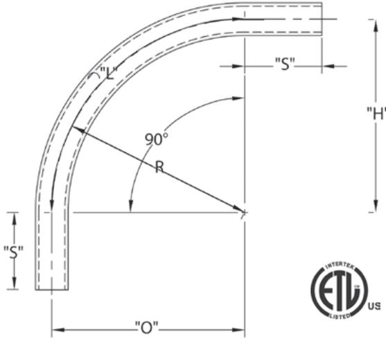
CANTEX Plain End Schedule 80 90-Degree Special Radius Elbows are used to change the direction of a conduit run by 90 degrees when special radiuses are needed.
