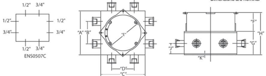
CANTEX ENS0507C is a 55.5 cu. in. ENT Slab Box with 1/2 & 3/4 inch Snap-In Connectors designed for use with electrical nonmetallic tubing (ENT) and standard electrical devices and switches in residential and light commercial applications.
