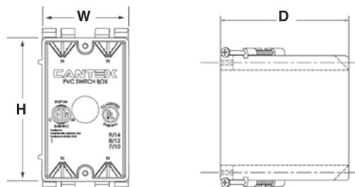
**EZ BOX® New Work, Nail-on, Switch and Outlet Box with Knockouts**
