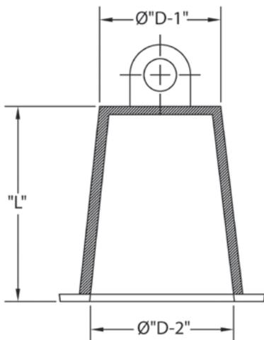
Poly Plugs with Pulling Eyes are designed for the temporary sealing of conduit to protect the duct from the effects of weather, job site debris, and animal damage. The molded pull-eye is used to secure excess pulling rope within conduit.
