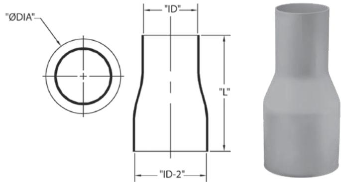
DB60 Swedged Reducer Bell to Plain is designed to transition conduit from one trade size to another trade size.
