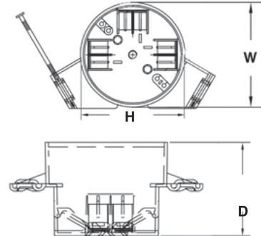
**EZ BOX® New Work, 20 cu. in. Ceiling Box with Hanger Bar and Wire Clamps**
