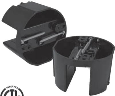
EZ12CF is a 12 cu. in. new construction (new work) ceiling fan box for residential and light commercial new construction (new work) applications. EZ12CF accommodates 3-1/2" and 2-9/16" mounting. CANTEX ceiling fan boxes are designed for easy, cost saving installation and they are constructed with durable polycarbonate for added resilience. The mounting screws are included.
