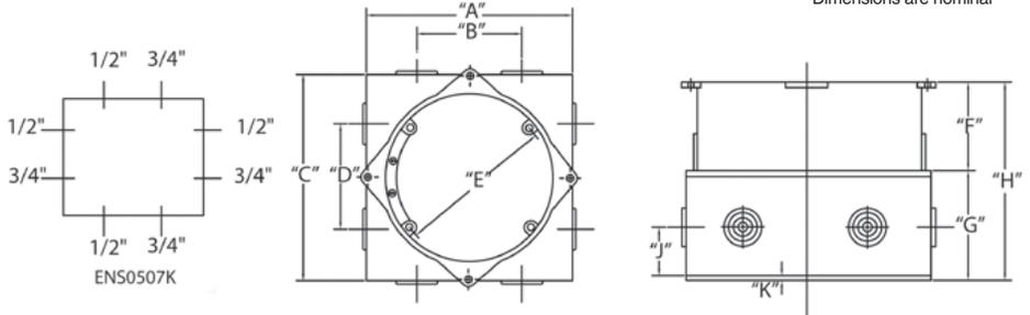
CANTEX ENS0507K is a 55.5 cu. in. ENT Slab Box with 1/2 & 3/4 inch Knockouts designed for use with electrical nonmetallic tubing (ENT) and standard electrical devices and switches in residential and light commercial applications.
