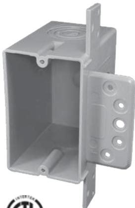
EZ BOX EN22SB is a 1-gang ENT box designed for use with electrical non-metallic tubing (ENT). This 22 cu. in. box is the largest capacity ENT 1-gang box available today. It features ample room for all necessary wiring. This box includes 1/2, 3/4 and 1 inch concentric knockouts to fit multiple sizes of ENT tubing and fittings.
