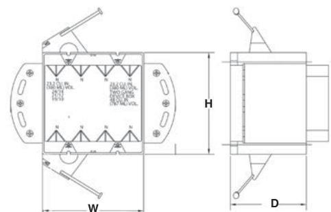
**EZ BOX® New Work, 2-Gang Switch & Outlet Box with Steel Stud Brackets & Express Clip®**
