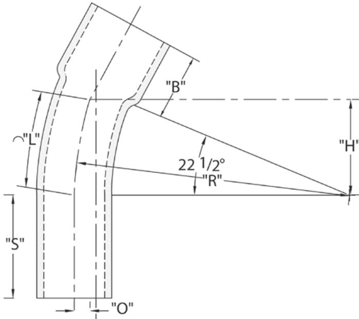
DB-60 Special Radius Bell End 22-1/2 Degree Elbows are used to change the direction of a conduit run by 22-1/2 degrees.
