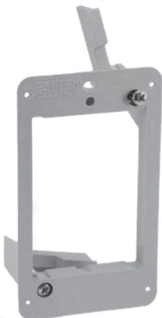
EZLV1-OW is a 1-gang EZ BOX old work, low voltage bracket used for low voltage installations in renovation (old work) applications. The backless design is great for the large or deep low-voltage wiring needed for communications and cable installations. It fits standard 1-gang faceplates.
