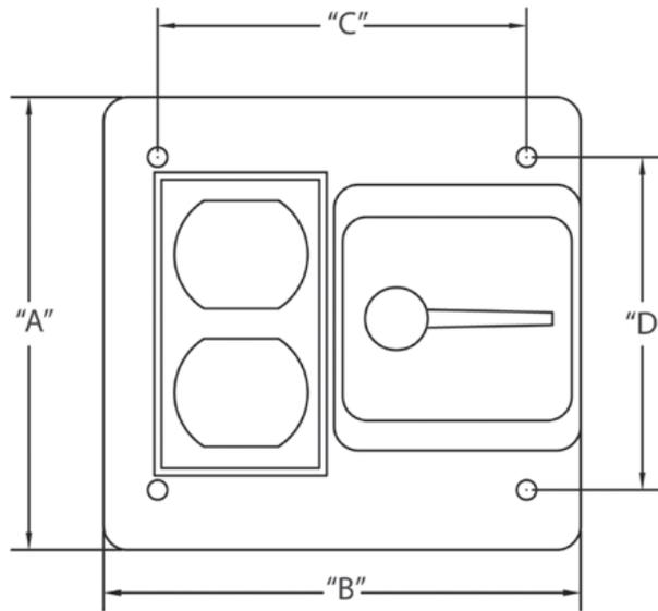
CANTEX 5133337 is a 2-Gang Weatherproof Duplex & Toggle Switch Cover designed for use with exposed weatherproof boxes.
