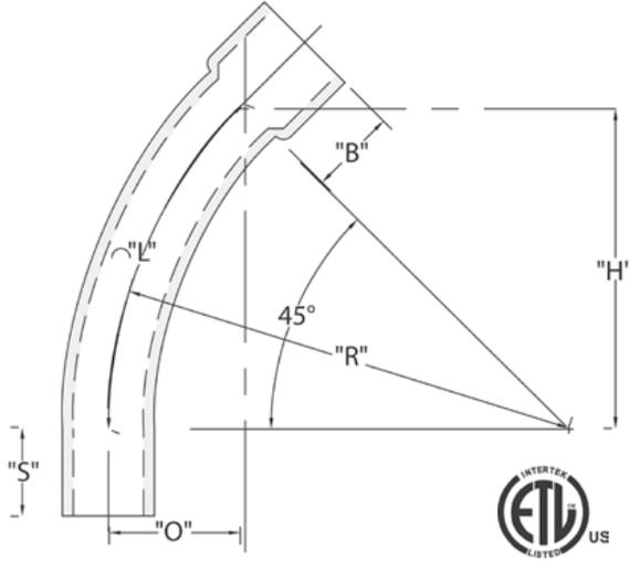
CANTEX Schedule 40 45-Degree Special Radius Belled End Elbows are used to change the direction of a conduit run by 45 degrees when special radiuses are needed.
