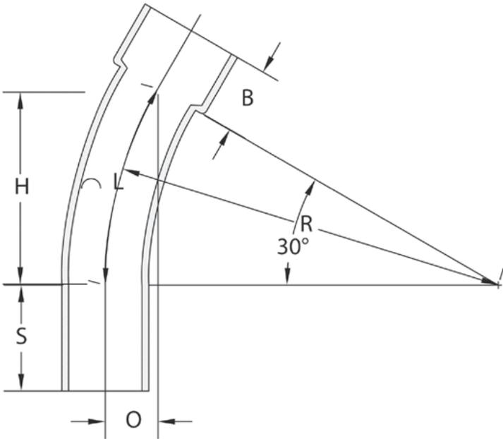
DB-60 Special Radius Bell End 30 Degree Elbows are used to change the direction of a conduit run by 30 degrees.
