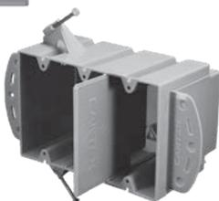
Divides multi-gang, maximum capacity boxes to allow for the installation of communication devices with standard switches or outlets. Fits 2 & 3-gang, maximum capacity, deep EZ BOXES.
