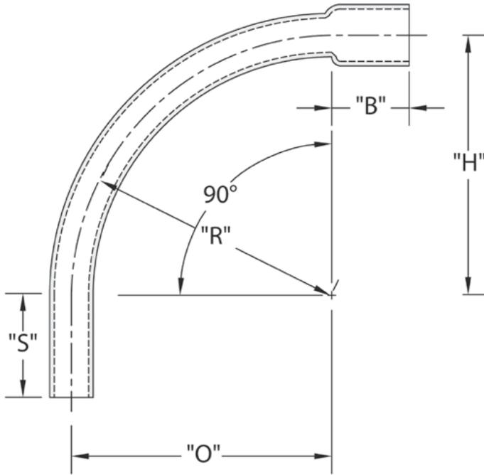
DB-120 Special Radius Bell End 90-Degree Elbows are used to change the direction of a conduit run by 90 degrees.
