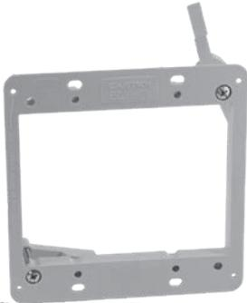
EZLV2-OW is a 2-gang EZ BOX old work, low voltage bracket used for low voltage installation in renovation (old work) applications. The backless design is great for the large or deep low-voltage wiring needed for communications and cable installations, and it fits standard 2-gang faceplates.
