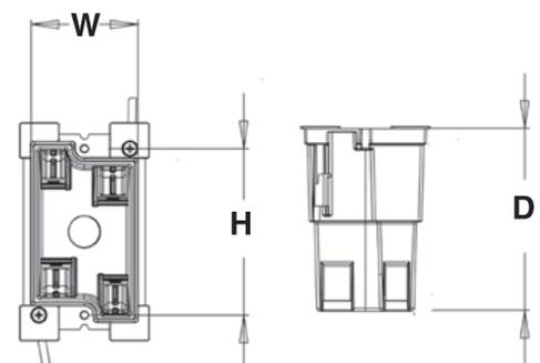
**EZ BOX® 2-Gang, 25 cu. in., Old Work Switch & Outlet Box w/ EZ Mount Flanges & Wire Clamps**
