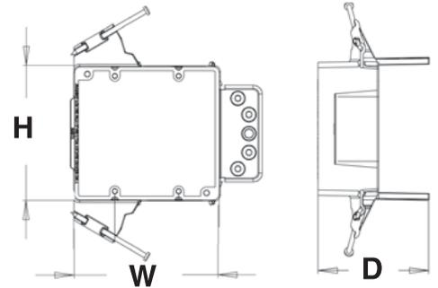
**EZ BOX® 2-Gang, New Work, Dual Voltage Bracket with Nails**
