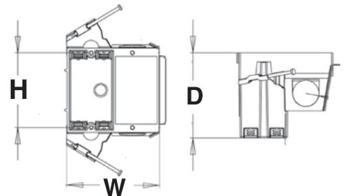
**EZ BOX® Low Voltage Divider for Use with Multi-gang Heavy Wall Boxes**
