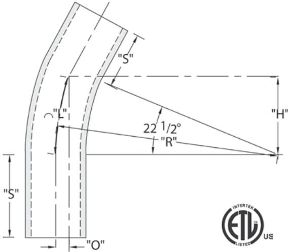
CANTEX 22-1/2-Degree Plain End Schedule 40 Special Radius Elbows are used to change the direction of a conduit run by 22-1/2 degrees when special radiuses are needed.
