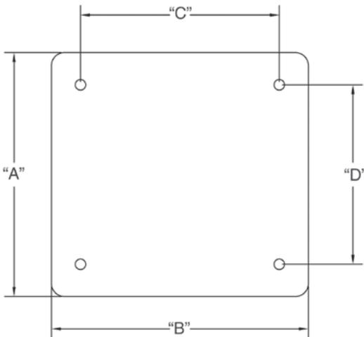
CANTEX 5133410 is a 2-Gang Weatherproof Blank Cover designed for use with exposed weatherproof boxes.
