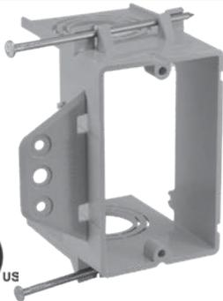
EZLV1-NWN EZ BOX is a 1-gang, new work, low voltage bracket with nails used for low voltage installations for new construction projects (new work) applications. The backless design is great for the large or deep low-voltage wiring needed for communications and cable installations, and it fits standard 1-gang faceplates. Round concentric knockouts allow for multiple fitting sizes.
