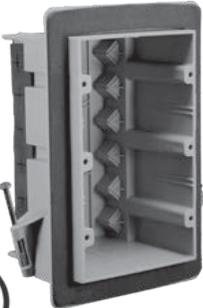
EZ54TN-RG is a 3-gang new work, vapor-proof EZ Box. It is an energy efficient electrical box for walls subject to unwanted air-flow. It eliminates air leaks with a solid drywall flange covered with a foam gasket and additional foam gaskets over self-clamping cable entry v-clamps, creating a vapor-tight seal and allowing no air to flow through the box. The EZ36DN-RG also features angled nails for EZ installation.
