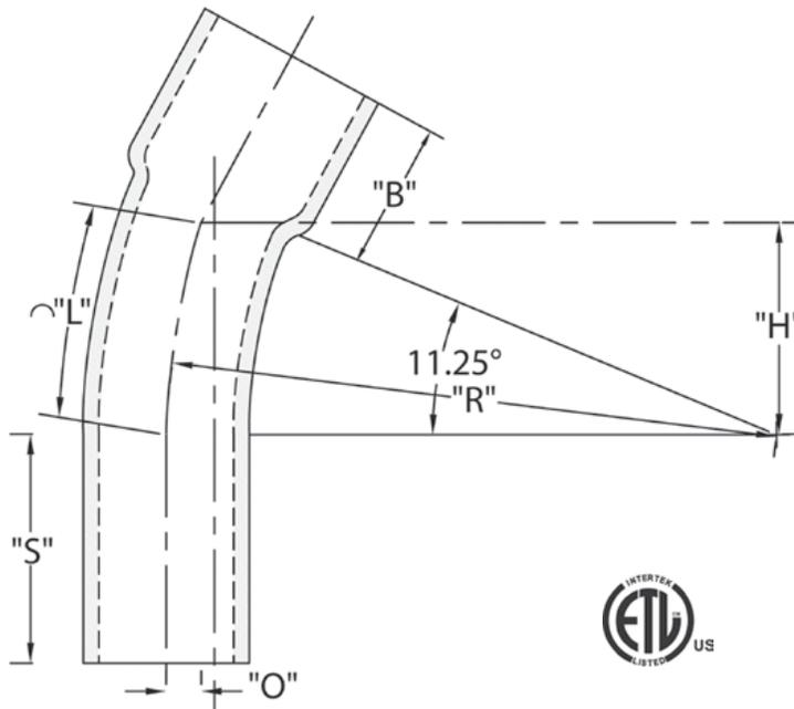
CANTEX Schedule 40 11 1/4 -Degree Special Radius Belled End Elbows are used to change the direction of a conduit run by 11-1/4 degrees when special radiuses are needed.
