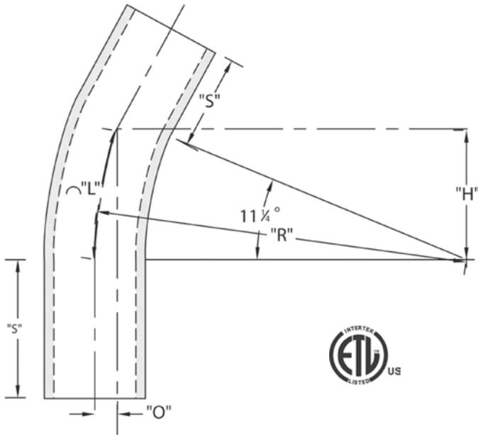
CANTEX 11-1/4-Degree Plain End Schedule 40 Special Radius Elbows are used to change the direction of a conduit run by 11-1/4 degrees when special radiuses are needed.
