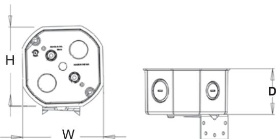
CANTEX EN20CB is a 20 cu. in. Octagon ENT Ceiling Box with an L-Bracket. It is for residential and light commercial ceiling fixture applications. It features an L-bracket for EZ and secure installation and 6 knockouts for multiple wiring options.
