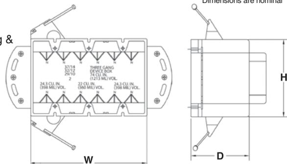
**EZ BOX® New Work, 3-Gang, Switch & Outlet Box with Screw Nails and Steel Stud Brackets**
