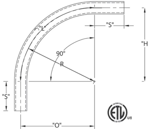
CANTEX Special Radius Plain End Schedule 40 90-Degree Elbows are used to change the direction of a conduit run by 90 degrees when special radiuses are needed.
