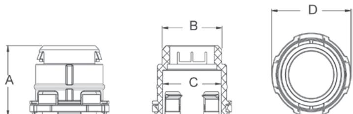
**ENT Slab Box with Knockouts**
