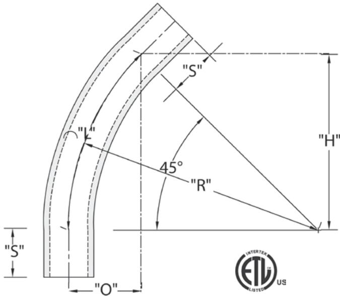
CANTEX Plain End Schedule 80 45-Degree Special Radius Elbows are used to change the direction of a conduit run by 45 degrees when special radiuses are needed.
