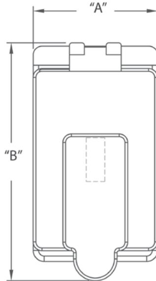
CANTEX 5133361 is a 1-Gang Weatherproof Switch Cover designed for use with exposed weatherproof boxes. For use in wet or damp locations.
