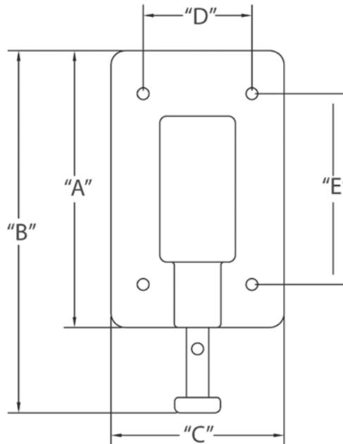
CANTEX 5133335 is a 1-Gang Weatherproof Plunger Switch Cover designed for use with exposed weatherproof boxes.
