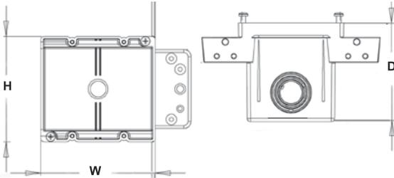
EZ BOX EN38DB is a 2-Gang 38 cu. in. ENT box designed for use with electrical non-metallic tubing (ENT). It features ample room for all necessary wiring and 1/2, 3/4 and 1 inch concentric knockouts to fit multiple sizes of ENT tubing and fittings.
