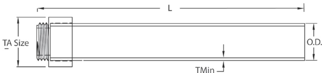
CANTEX PVC Schedule 40 & 80 and DB-120 Service Risers with a 45° bend provide permanent protection for underground services where they emerge from the ground. The 45° bend eliminates the cost, time and labor to install a separate elbow. Formed from CANTEX Schedule 40 & 80 and DB-120 conduit that are resistant to UV light, their use assures compliance with Article 300-5 of the National Electrical Code.
