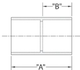
Schedule 40 Long Line Center Stop Couplings are used to repair or join lengths of conduit/ pipe together with two solvent weld socket ends.
