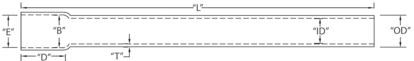
Note: 20' length available on request with the exception of the 1/2 inch conduit sizes. Schedule 40 conduit complies with federal and military specifications by conforming to UL 651.
