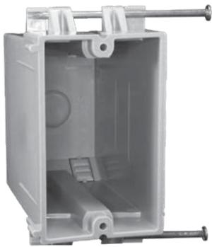
EZ22SN-HW is a 1-gang, 22 cu. in., heavy wall EZ BOX that is ideal for new work applications for residential and light commercial projects where an even more durable box is preferred. The harder shell is designed to resist flexing and hold its shape in extreme conditions. EZ22SN-HW also features enhanced angled nails for easy mounting between studs and knockouts for EZ wiring.
