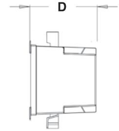
**EZ BOX® 3-Gang, Old Work, 55 cu. in. Switch and Outlet Box with EZ Mount Flanges and Wire Clamps**
