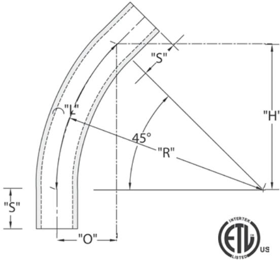
CANTEX 45-Degree Plain End Schedule 40 Special Radius Elbows are used to change the direction of a conduit run by 45 degrees when special radiuses are needed.
