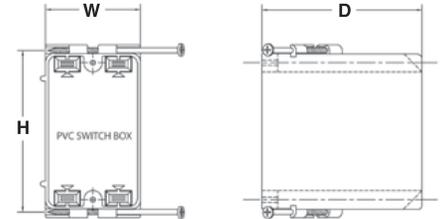
**EZ BOX® New Work Switch and Outlet Box with Screw-Nails**
