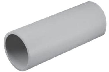
Schedule 40 Long Line Couplings with No Center Stops are used to repair or join lengths of conduit pipe together with two solvent weld socket ends.
