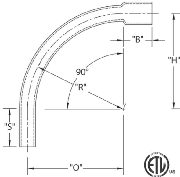
CANTEX Belled End Schedule 80 90-Degree Special Radius Elbows are used to change the direction of a conduit run by 90 degrees when special radiuses are needed.
