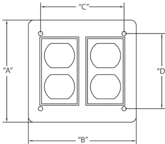
CANTEX 5133347 is a 2-Gang Weatherproof Double Duplex Cover designed for use with exposed weatherproof boxes.
