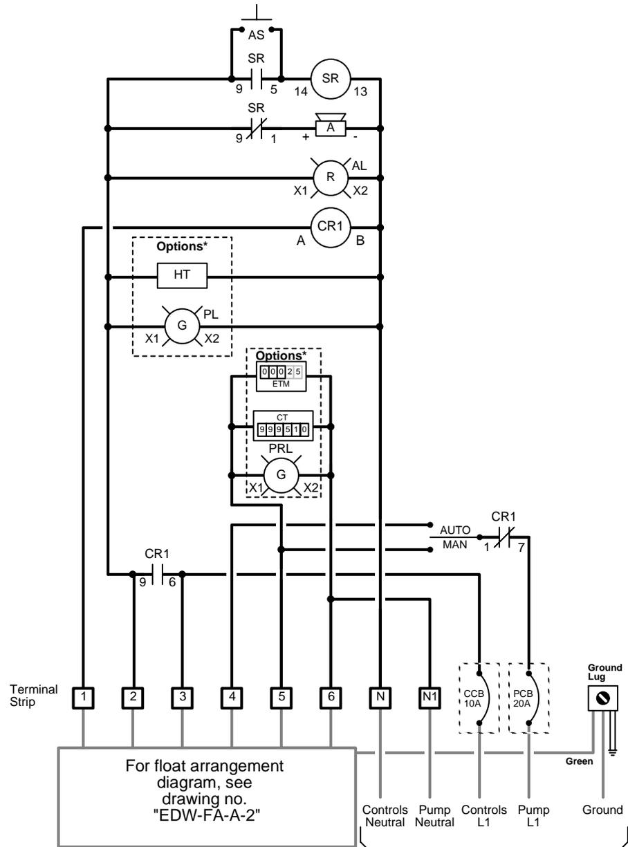
NOTE: Motors must have internal overload protection
