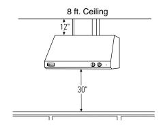
**8 ft. ceilings:** When the hood is installed 30" above the cooking surface and there is no soffit or upper cabinetry, order one 12" duct cover accessory.
