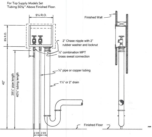
PLUMBING ROUGHING-IN MEASUREMENTS FOR SPACE SAVER WASHING MACHINE SUPPLY AND DRAIN MODEL FB 150 & FB 200
